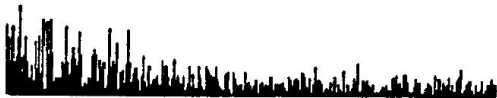
Fig. 4: Computed amplitude spectrum (zero frequency at left) of a long one-dimensional section of the noise shown in Fig. 2. The spectrum is not bandpass.
